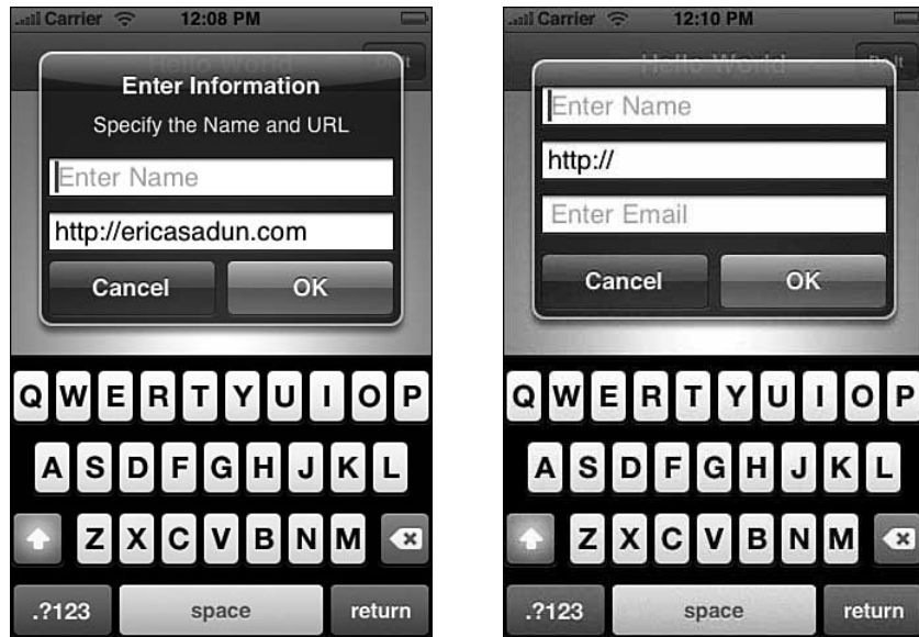
Figure 4-4 Using careful space management and omitting the title and body text, you can add up to three text entry fields to a UIAlertSheet at once. You probably want to limit your UIAlertSheets to one or two text fields.
