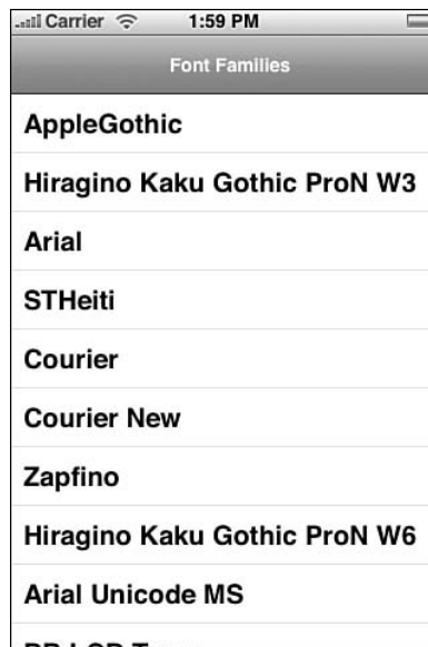
Figure 5-1 It's easy to fill a UITableView with cells based on any array of strings. Here, the font family list from the UIFont class is listed. When tapped, the font chosen will update the title bar font.
