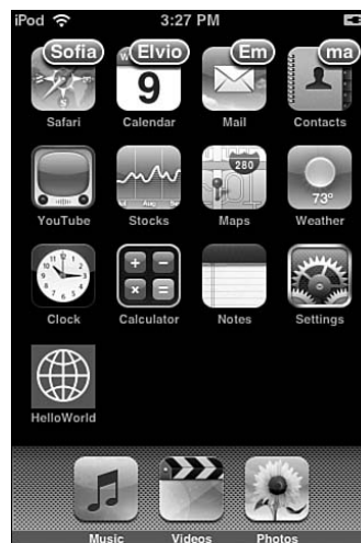
Figure 4-12 Application badges appear as small, red containers on the top-right corner of an application's icon.
