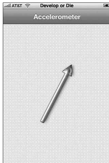
Figure 9-4 A little math recovers the “up” direction by performing an arctan function using the x and y force vectors. In this sample, the arrow always points up, no matter how the user reorients the iPhone.
