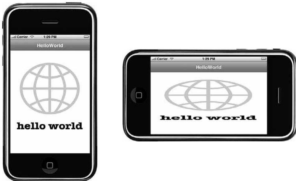
Figure 1-3 UIViewController controllers can automatically handle view orientation changes by scaling their subviews. When working with images, you'll probably want to catch orientation changes and swap out a landscape-friendly version rather than accept the squeezed aspect shown here.
