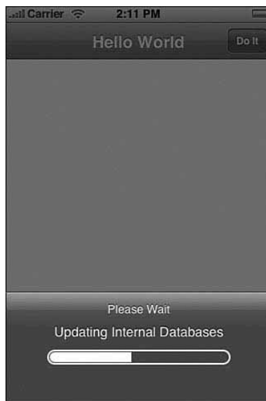
Figure 4-8 Use UIProgressView instances to track progress over an extended delay. Adding them to a UIActionSheet simplifies their presentation and dismissal.
